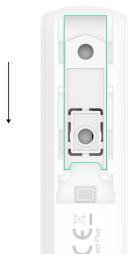
2. If you are using a large magnet, remove the SmartBracket mounting panel from it by slightly pushing and pulling it down as shown in the previous step. If you are using a small magnet, disassemble its enclosure by prying up the back with a flat object. Use a slotted screwdriver for this.
