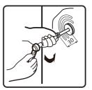
Push two transportation bolts on horizontal direction inward and loose transportation bolt.
