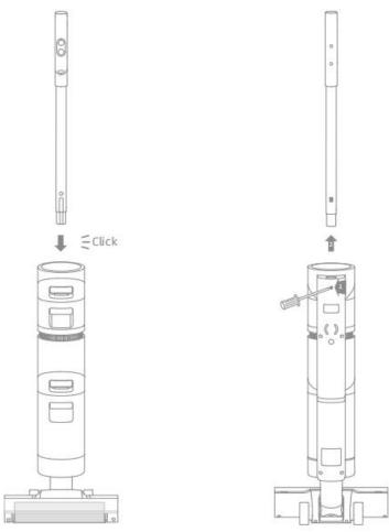
Note: To disassemble the handle, please use a hard object to reach into the hole on the back of the vacuum to press the contacts, and at the same time, pull the handle upwards.
