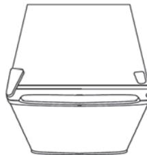
Check that the door is aligned horizontally and vertically and that the seals are closed on all sides before finally tightening the upper hinge. Re-adjust the leveling feet.
