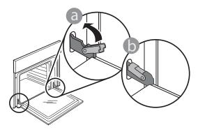
**5.** Try closing the door and check to make sure that it lines up with the control panel. If it does not, repeat the steps above: The door could become damaged if it does not work properly.
