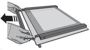
**2.** Lift and firmly hold the inner glass with both hands, remove it and place it on a soft surface before cleaning it.
