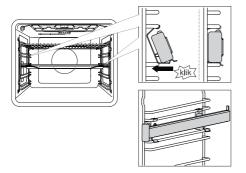
The click-on pull-out guide can be inserted into any space between two wire guides.
