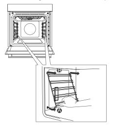
${\sf A}$  Hold the guides by the bottom side and pull them towards the center of the oven cavity.
