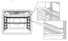
In case of wire guides, always insert the wire rack and the baking tray into the slot between the upper and lower part of each guide level.
